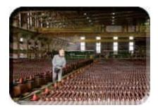
1. The copper anodes are placed in cells between stainless steel blanks submerged in electrolyte.
