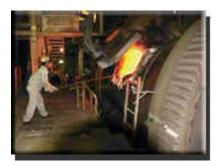
Refined copper from Anode furnace is cast continuously into copper strip by a Hazelett Twin Belt Caster. This continuous copper strip is cut into anode pieces by a hydraulic shearing machine
