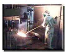
Matte and flux (limestone) are reacted with oxygenenriched air to form blister copper and then separated from the slag by difference of specific gravity. Slag (Cu14%) is returned to Sfurnace, and blister copper is siphoned out and forwarded to Anode furnaces.
